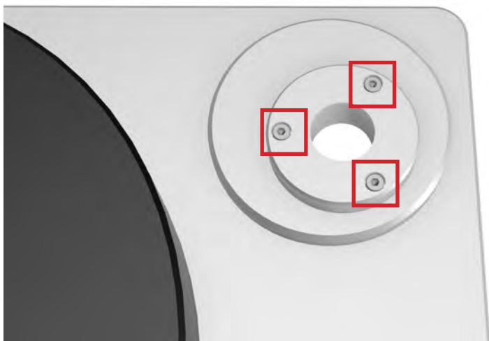
Pic. 8: Mounting the clamping ring
